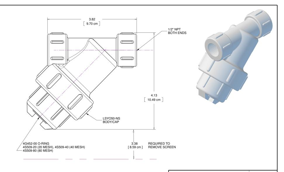
MATERIAL - GLASS REINFORCED POLYPROPYLENE BODY AND CAP 304 STAINLESS STEEL SCREEN VITON O-RING BEE VALVE, INC
